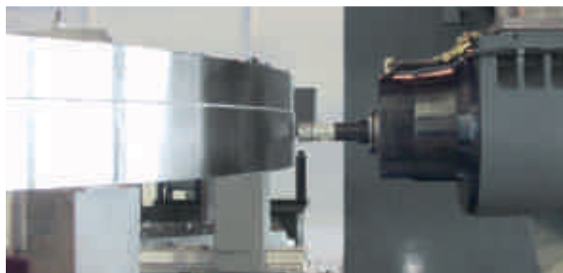
Horizontal ring machining with 2-axis tilting head and a rotary table
