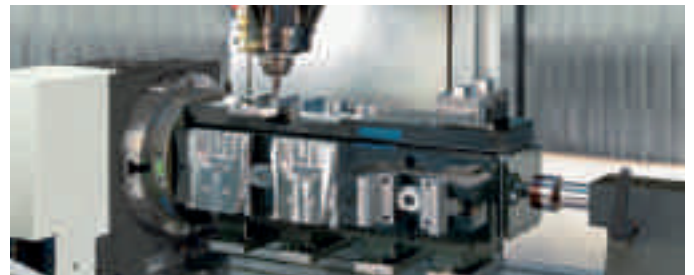
Rotary table with tailstock and swivel bridge for mechanical multiple clamping system
