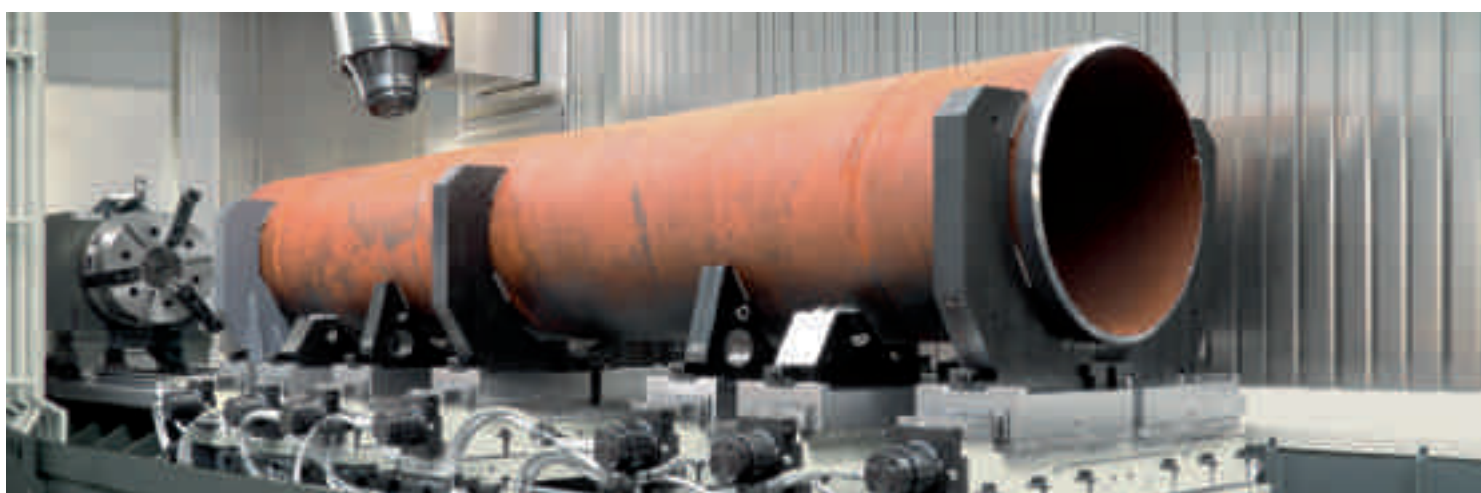
Manual or NC-driven pre-centering and presetting of the clamping elements for the next workpiece diameter
