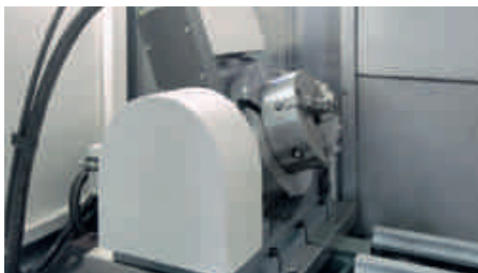
2-axis NC-tilting rotary table from AXA with continuous 360° round axis and tilting axis from 0° to 90°
