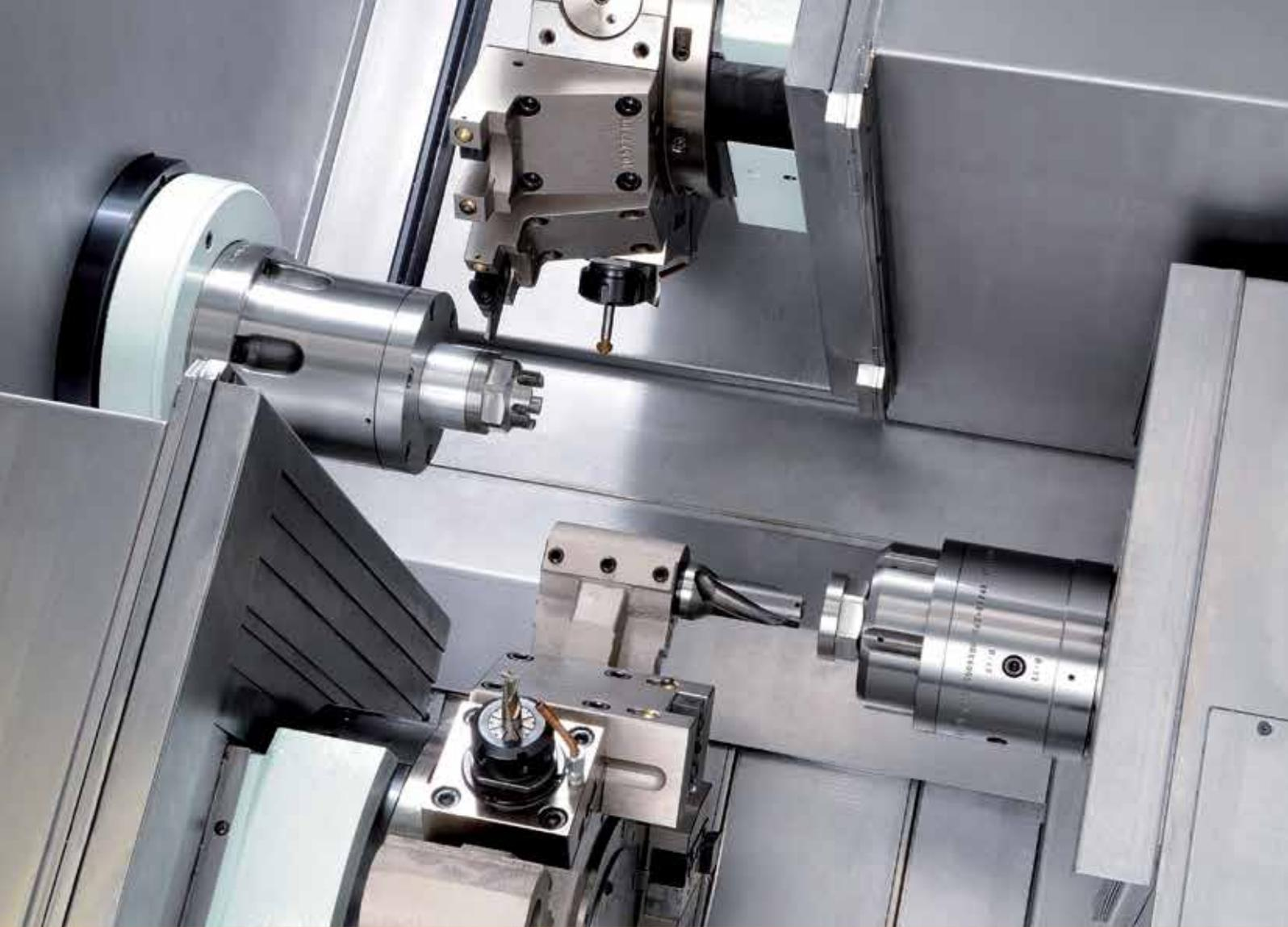
**Double-spindle and double-turret turning centres featuring two Y-axes:
