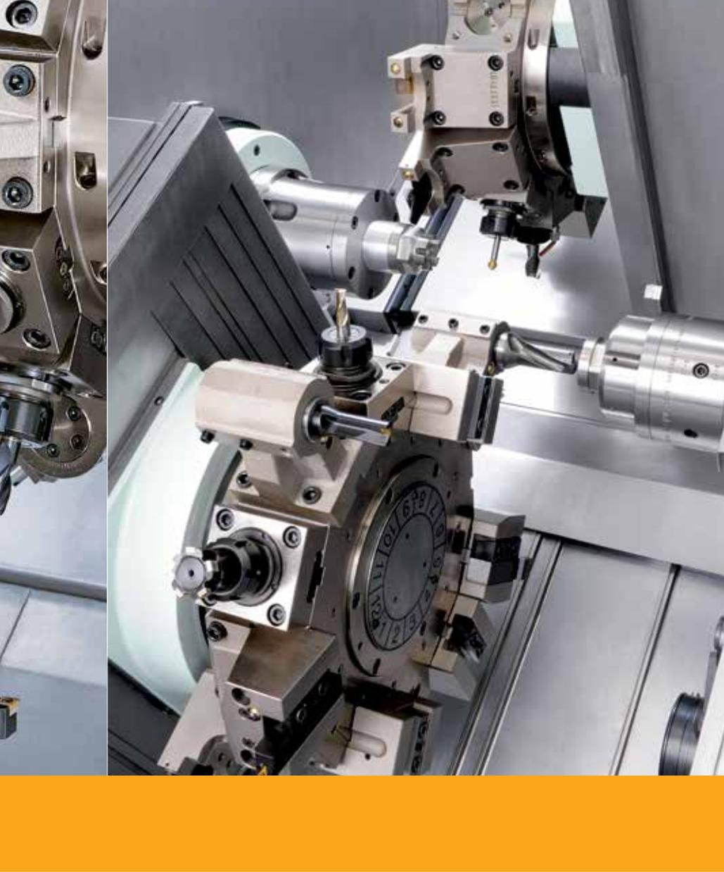
The position of the turrets and the sub-spindle featuring a double movement (longitudinal and transversal) enables reliable and flexible machining operations on both spindles. The main advantages are:
