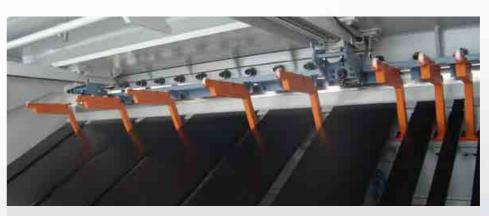
Lever type pneumatic sheet support system (optional) Avoids hanging down the wide and thin sheets via pneumatic arms support and provides more precise cuts.
