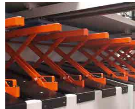
X type pneumatic sheet support system (optional) Protects sheets hanging down and improves precision for long and thin sheets cutting. Difference of this system than others is moving down parallel together with cut sheet and supports the sheet during entire cutting process.
