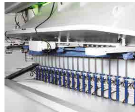
Anti-Twist system. (option) Anti-Twist system prevents cutting sheet material from twisting in narrow and strip cuttings by holding straight during the cutting process against to blade movements.
