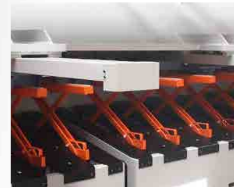
Return to Sender System (optional) Precisely cut plate via the assistance of X type pneumatic sheet support system at the rear is being returned to the front of the machine by this system.
