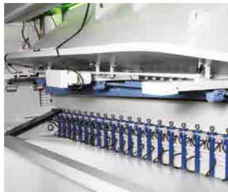
Anti-Twist system. (option) Anti-Twist system prevents cutting sheet material from twisting in narrow and strip cuttings by holding straight during the cutting process against to blade movements.
