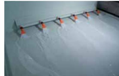
**Chips Flushing Nozzles**
