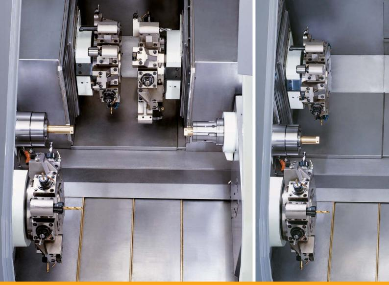
Double-spindle turning centres featuring three turrets and three Y-axes: high productivity in machining complex par
