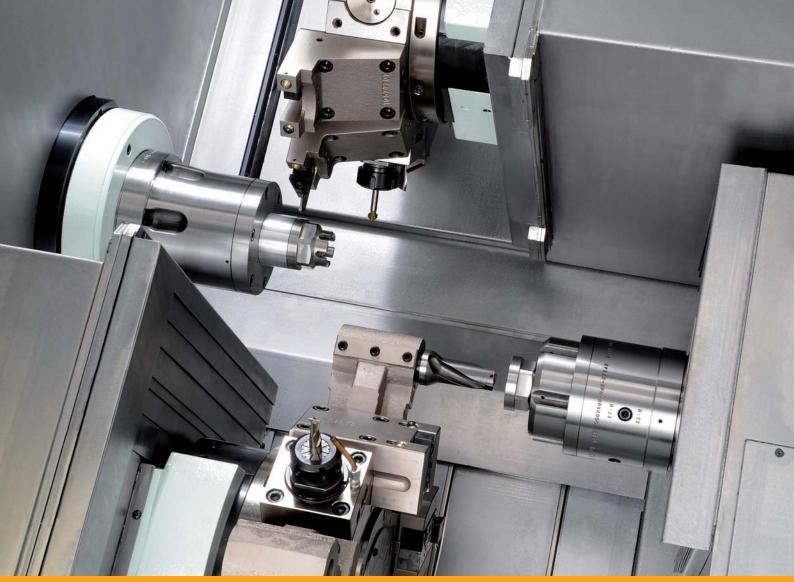
Double-spindle and double-turret turning centres featuring two Y-axes: high productivity in machining complex part
