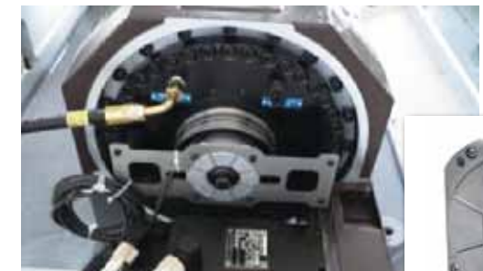
High precision angle encoder fit on A-axis and C-axis.
