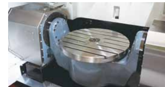
Hydraulic and pneumatic power supplied from table center.
