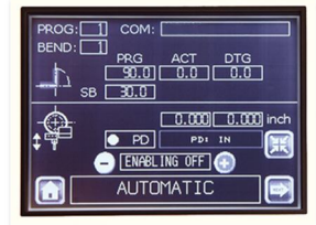
AUTOMATIC Displays current program, information, programmed angle, bend sequence, distance to go & actual position.
