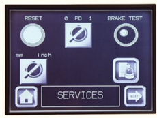
SERVICES Gateway to all machine services. Select multiple languages, monitor and adjust machine settings, view detailed alarm information, reset emergency stop, set pressure die ON/OFF and troubleshoot machine functions.
