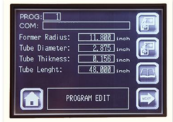
PROGRAM Select, enter and store program information, former radius, tube diameter, wall thickness and tube length.
